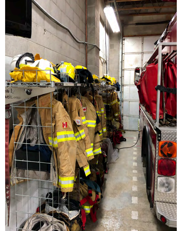
PPE storage located with apparatus bays - limiting access to and around vehicles. this also places gear with the same space as the vehicles which exposes them to further contaminants once they have been cleaned and does not allow for them to dry effectively.
