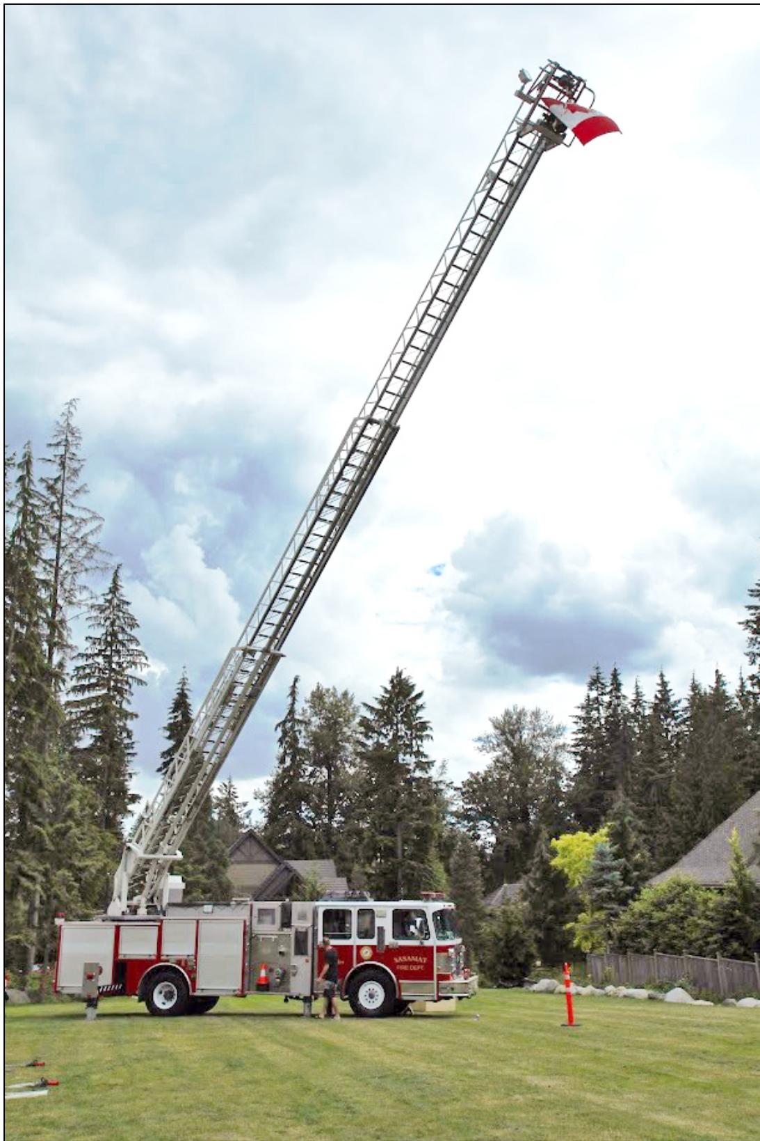
SVFD's Ladder Truck #7 — 75-Foot Ladder Fully Extended
